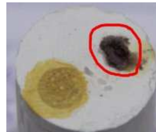
Figure 17 - iodine test on a piece of spent grain from experiment 33 (0.95 mm) (circled in red)
