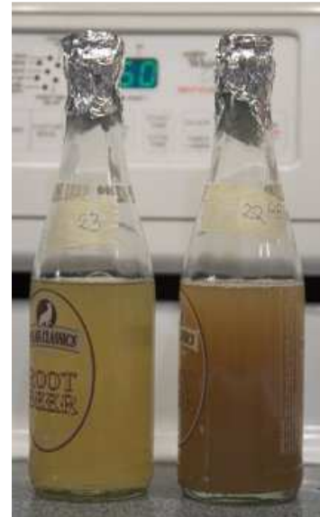
Figure 14 - A comparison of the wort colors after a 15 min boil for experiments 23 (pH 5.5) and 22 (pH 6.5). The darker color of the higher pH wort is remarkable. It is a result of the stronger maillard reactions at the higher pH.
